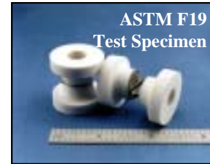
Al-500 alumina brazed with Ag-3.4Hf & 0.25 mm Kovar™
